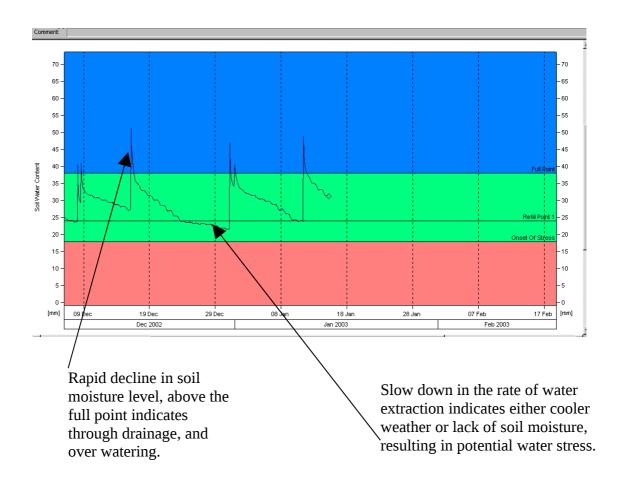
There are a wide range of sensors available to measure soil water content or soil tension that can be used to develop and manage irrigations. These can be simple manual type of sensors or probes where users must go into the field and take readings, data loggers where the information from the sensors is continuously recorded and systems that can transmit readings from the field to a computer with small radio units.
