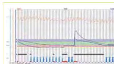
Figure 1. Data of a typical cycle for a field showing soil moisture decreasing (blue line) and the system enabling irrigation (black line) when the low set point is reached. Irrigation (blue bars) and rain (red tag) then puts the soil moisture above the high set point and irrigation is again disabled and so on. Note that rain at the end of the irrigation cycle sent soil moisture to field capacity.
